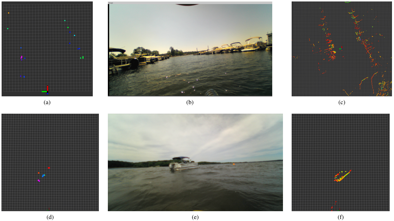
Fig. 2: Results from different sensors mounted on the ASV. (top row) Lake Murray, SC, USA: (a) Radar data (crowded); (b) Camera view (crowded); (c) Velodyne LIDAR data (crowded); (second row) Lake Wateree, SC, USA: (d) Radar data (single boat detected); (e) Camera view (single boat detected); (f) Velodyne LIDAR data (single boat detected).
