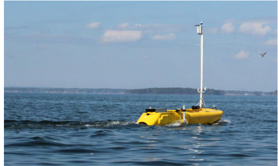
Fig. 1: Autonomous Surface Vehicle collecting bathymetric and water quality data at Lake Murray, SC, USA.
