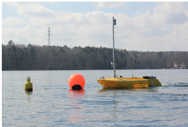
Fig. 1: Autonomous Surface Vehicle collecting bathymetric and water quality data around a permanent sensing station.
